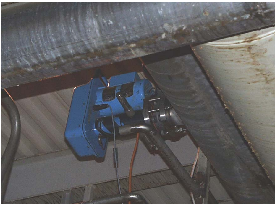
KPM's rotary consistency transmitter at bleach plant of the Kemi pulp mill.
